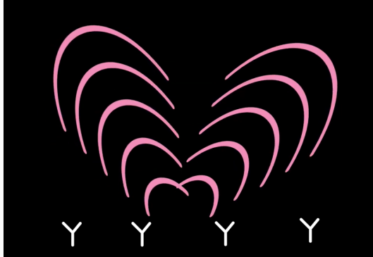
Figure 3: Antenna arrays are generating multiple beams targeted to multiple users and can steer them independently of each other using phase shifting
